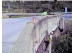
conducted a non-destructive live-load test of a 1920's reinforced concrete bridge in Royalton, Vermont. Strains were monitored
